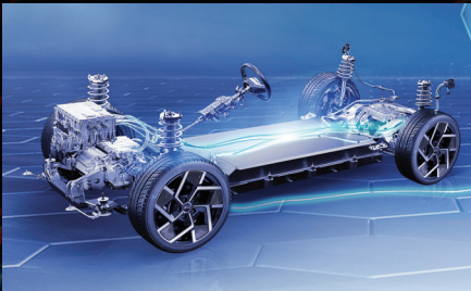
Safety - E-Platform 3.0 With The Cell-to-Body (CTB) Structure
